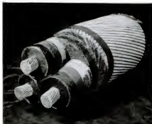
CROSS SECTION shows three conductors which carry current. There are 61 copper strands in each.
